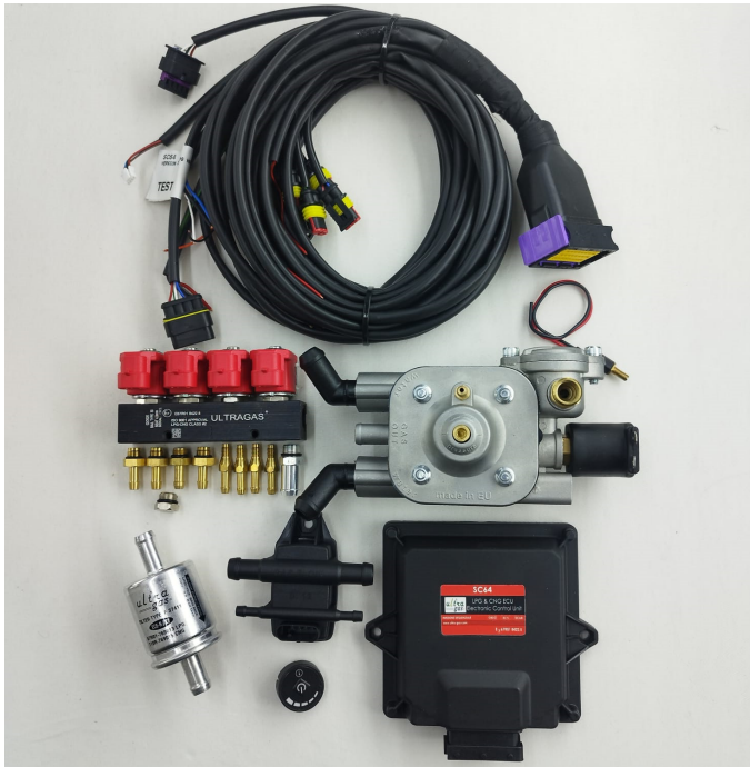
4 CYL UG64-M ECU SET 24 pin) No OBD II TIGER-X Regulator 200 RAIL Type Injector 2 or 3 OHM + LPG Filter
